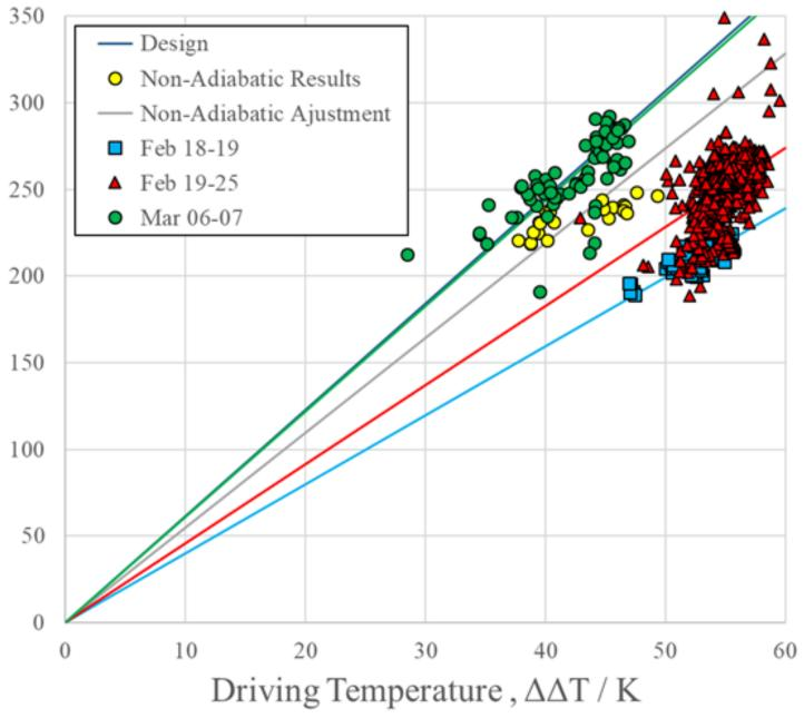
$\Delta \Delta T = R \cdot (t_{eva} - t_{con}) - (t_{abs} - t_{gen})$
