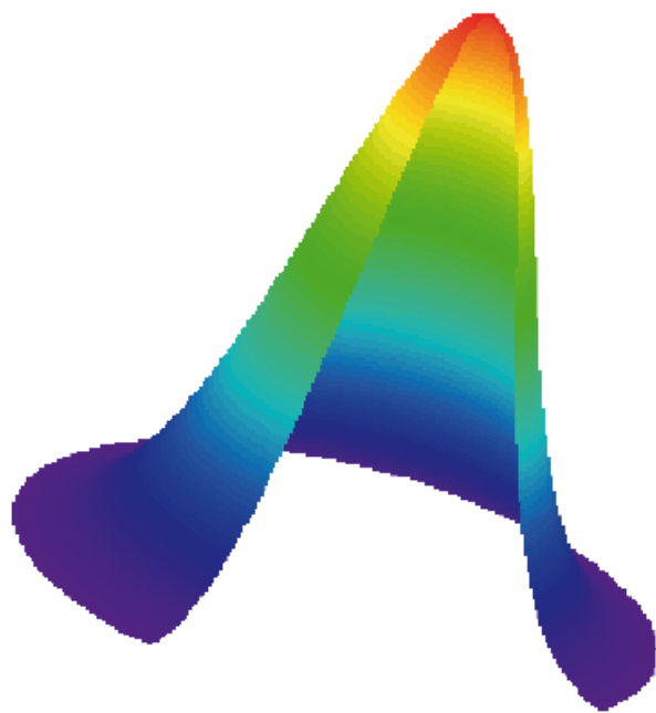
Figure 2a. The three-dimensional field-intensity distributions on the rectenna for the Gaussian beam.
